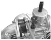
6 . With an adjuster, adjust the free play at the throttle grip to be approximately 5 mm.
