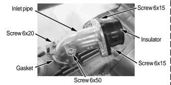
Put the carburetor into the insulator, and hold it by tightening a band. Attach an air filter, and hold it by tightening a band.
