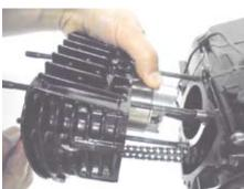
O Align the guide roller with the cylinder mounting hole and temporarily tighten the guide roller bolt/new sealing washer.
