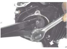
O Remove the tensioner rod oil filler bolt.
