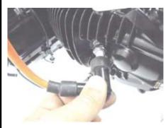
O Prepare the pan, remove the drain bolt/ sealing washer, filler cap, and drain the engine oil.
