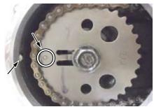
O Hold the cam sprocket (with a universal holder) and tighten the cam sprocket bolt / washer to the specified torque.
