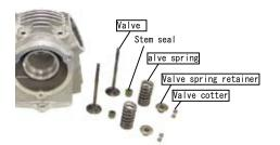
Check each valve for bending, baking, and damages.
