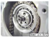
O Fix a cam shaft circlip of the kit, and fix the cam shaft. At this stage, set the location of ring end gap of the circlip not to meet the notch on the cylinder head cam hole.
