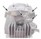
O Apply engine oil a little to a left-side-cover O-ring of the kit and fix it to the left side cover. Then fix them to the cylinder head with two 5x15 cap screws and with a 5x10 cap screw of the kit and tighten them to the specified torque. (Be careful of the location of screws.)
