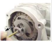
O Tighten the adjusting nut to the specified torque.
