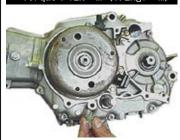
O With reference to the service manual, mount the engine on the frame
