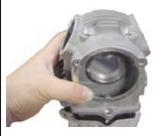
O Fix the cam chain so it will not fall into the crankcase.
