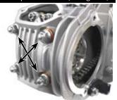
O Tighten the two side bolts of the cylinder head alternately in several steps to the specified torque. Attach guide roller bolt (with sealing washer) and tighten it to the specified torque.
