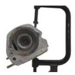
• Strike lightly the end of valve stems a few times so the valves and cotters fit together well.
