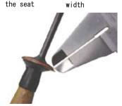
Service Limit: IN:1.5mm more repair or replace the cylinder head EX:1.7mm more repair or replace the cylinder head
