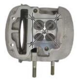
Service limit: If the distortion is over 0.05 mm, rectify or replace the cylinder head.
