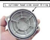
O Apply engine oil a little to a inspection cover 0-ring, and fix it to the inspection cover, and fix the inspection cover with socket cap screw (5x12) and tighten them to the specified torque
