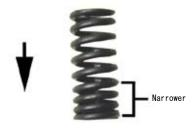
Compress the valve spring with a valve spring compressor.
