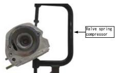
Use a magnet to remove the cotter if it does not come off easily.
