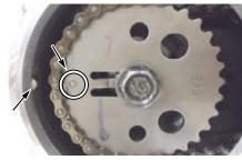
O Fix the cam sprocket with a universal holder, remove the cam sprocket bolt/ washer, and remove the cam sprocket.
