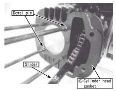
O From here on, please assemble the cylinder head following to the "Super Head 4V+R" installation manual.
