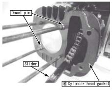
O Place the cam chain through the cylinder head and install the cylinder head.
