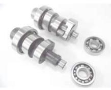
O Remove the de-comp parts from the stock camshaft. Attach the decompression parts to the (9) camshaft in the same way. % Caution: direction of the washer.
