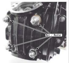
O Tighten the four cylinder head nuts diagonally in several steps to the specified torque.
