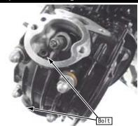
O Make sure that the alignment mark on the flywheel matches the alignment mark on the crankcase, and align the cam sprocket so that the "O" mark on the cam sprocket aligns with the protrusion on the cylinder head. Attach the cam chain and align the protrusion of the cam sprocket with the groove of the camshaft.
