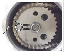
O Fix the cam sprocket with a universal holder, remove the cam sprocket bolt/ washer, and remove the cam sprocket.
