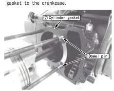
O Apply engine oil to the piston ring and let it blend in Apply engine oil after cleaning the inner circumference of the ① cylinder.
