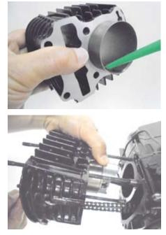
O Align the guide roller with the cylinder mounting hole and temporarily tighten the guide roller bolt/new sealing washer.
