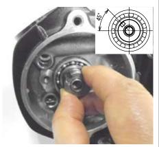
• Next, rotate groove to the exhaust side at about 45 degrees and remove the cam crest and de-comp mechanism with the shape of the head.
