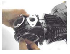
O Install x4 washers, head nuts and x2 cylinder head side bolts.
