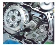
• Attach the O-ring(12mm) to the oil through nut and apply a engine oil to the O-ring.
