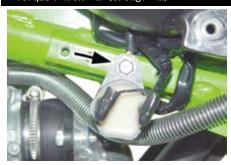
O Fit an inlet pipe into the circled bolt holes on the cylinder head.
