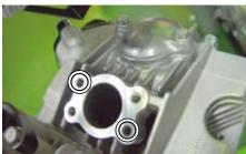
O Put a gasket between the cylinder head and an inlet pipe, and fix it with 6x20 socket cap screws.
