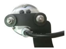
O Remove the left and right bolts at the bottom of the headlight unit.
