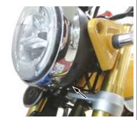
O Remove the headlight unit from the bottom and remove the top nail.
