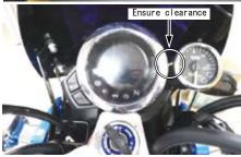
O Refer to the photo (use the play) in the meter mounting area to create a gap between the genuine meter and the DN meter then use the genuine bolts to secure the bracket. Place the wire on the meter side through the headlight case.
