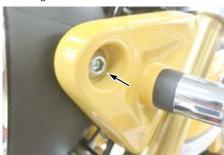
O Remove one bolt in the headlight case.
