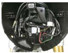
O Move the headlight case and remove the genuine meter cover mounting bolt.
